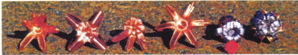
The bullets tested in gelatine. From left a SMJHP-C (bone and gel), 90gr Peregrine SD bullet, SME-C that lost some of its petals, the SMJHP-C, Hornady Critical Duty and Winchester Defender.
