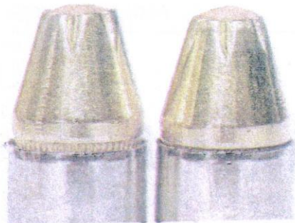
The cartridge on the left is the standard factory load. The one on the right has the bullet seated slightly deeper to eliminate feeding problems in my pistol.
