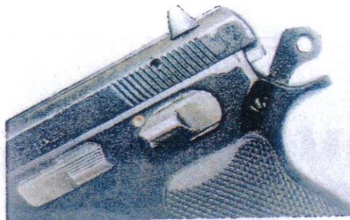
The slide would not fully close when feeding Critical Duty cartridges from the magazine.
